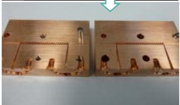
First samples of the fabricated FWG are shown in the figure beside. The small section of the waveguide requires high precision CNC milling to be realized with tolerance in the micron range. The beam optics is also in advanced fabrication phase.
